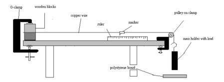
**Uncertainties in measurements** To measure the Young modulus all that is necessary in principle is to measure the extension of a sample for a given force and then to calculate the To find E, a graphical method is usually used. Since:
