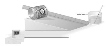
The temperature of the liquid is varied using a water bath. The viscosity of the liquid will affect the rate at which the tin or bottle rolls down a fixed ramp.
