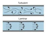
Laminar flow is an important consideration in fluid motion. The uplift on an aeroplane's wings is dependent on laminar flow, and passengers experience a rocky ride when turbulent conditions are encountered. Similarly, the drag forces on a motor car are affected by turbulence, and wind tunnels are used to observe the nature of the airflow over prototype designs.
