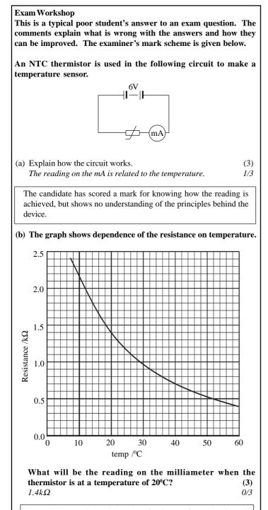
The pupil has merely read the value of resistance from the axis, and not used V = IR to calculate the current.
