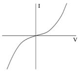
On the I/V plot the resistance is the inverse of the gradient, i.e. the resistance is **decreasing**. This is because as V increases, the thermistor gets hotter.
