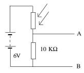
The resistance of the bottom resistor is fixed at, say,  $10 \text{ k}\Omega$ . The LDR in the top part of the potential divider has a resistance that will vary depending on the light intensity. It may be from the order of  $1M\Omega$  in low light, to  $1k\Omega$  in higher light levels. In strong light, the resistance of the LDR will be about  $1k\Omega$ , hence the P.D. between A and B will be about (10k/11k) 6V i.e. not far off 6V.
