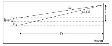
the laser – which could be the opposite wall – and maxima and minima are observed as clear patches of bright light and darkness. These represent the positions where the waves are exactly in phase or exactly out of phase respectively – just as seen with the ripple tank interference experiment above. This equation describes the relationship between the various measurements which may now be taken, where:
