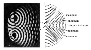
The ripple tank demonstrates wave properties in water waves – which have wavelengths large enough to be seen clearly. However, once the effects of wave properties have been understood, those *effects* can be recognised, observed and investigated using other types of waves even when the wavelengths involved are either too large or too small for the individual *waves* to be seen.
