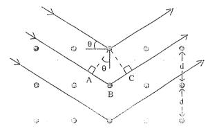
The receiver will measure an interference maximum when the extra distance travelled by the second ray is a whole number of wavelengths:
