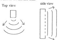
Diffraction from the narrow horizontal aperture fans the sound out across the half.
