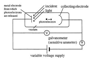
The circuit above shows a photocell. As the voltage of the supply is increased, more and more electrons are repelled back, and the galvanometer reading falls. Only the fastest electrons reach the collecting electrode. When the supply voltage reaches a value known as the stopping potential, even the fastest electrons can not reach the collecting electrode and the current falls to zero.
